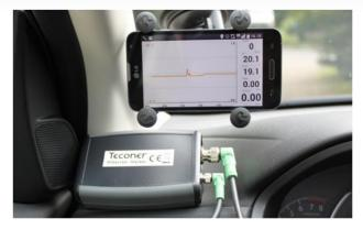
Photograph of the user interface with temperature measurements and the Bluetooth communication enclosure inside the vehicle.
